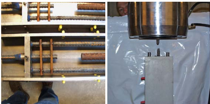
Samples for testing of pullout strength.
