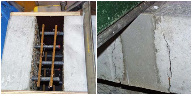
Even with lap lengths of 80 mm for ø12 reinforcing bars, the joint will be the strongest part of the element.
