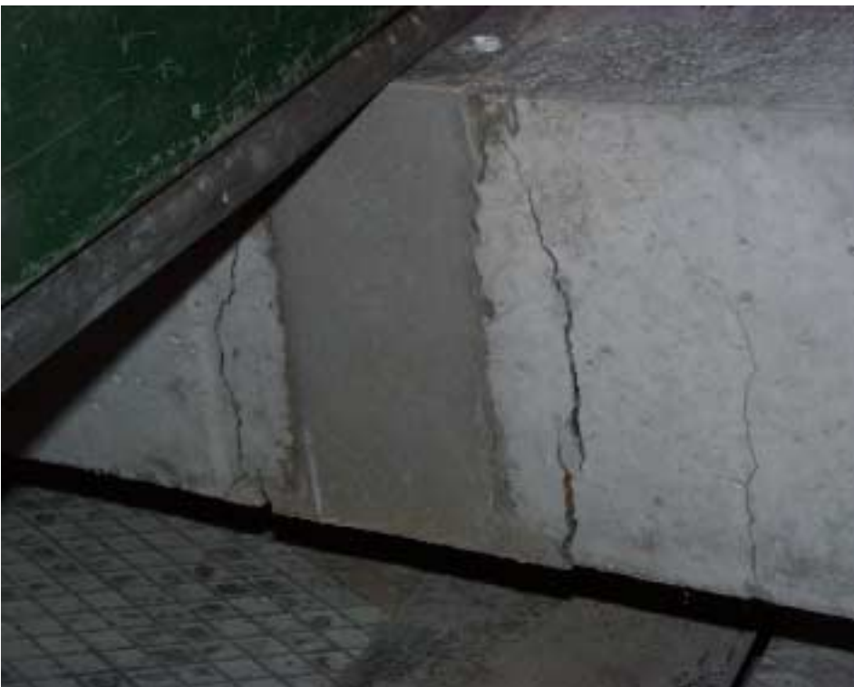
Simple joint with 12 mm bars and a width of 100 mm. The beam fails away from the joint.
