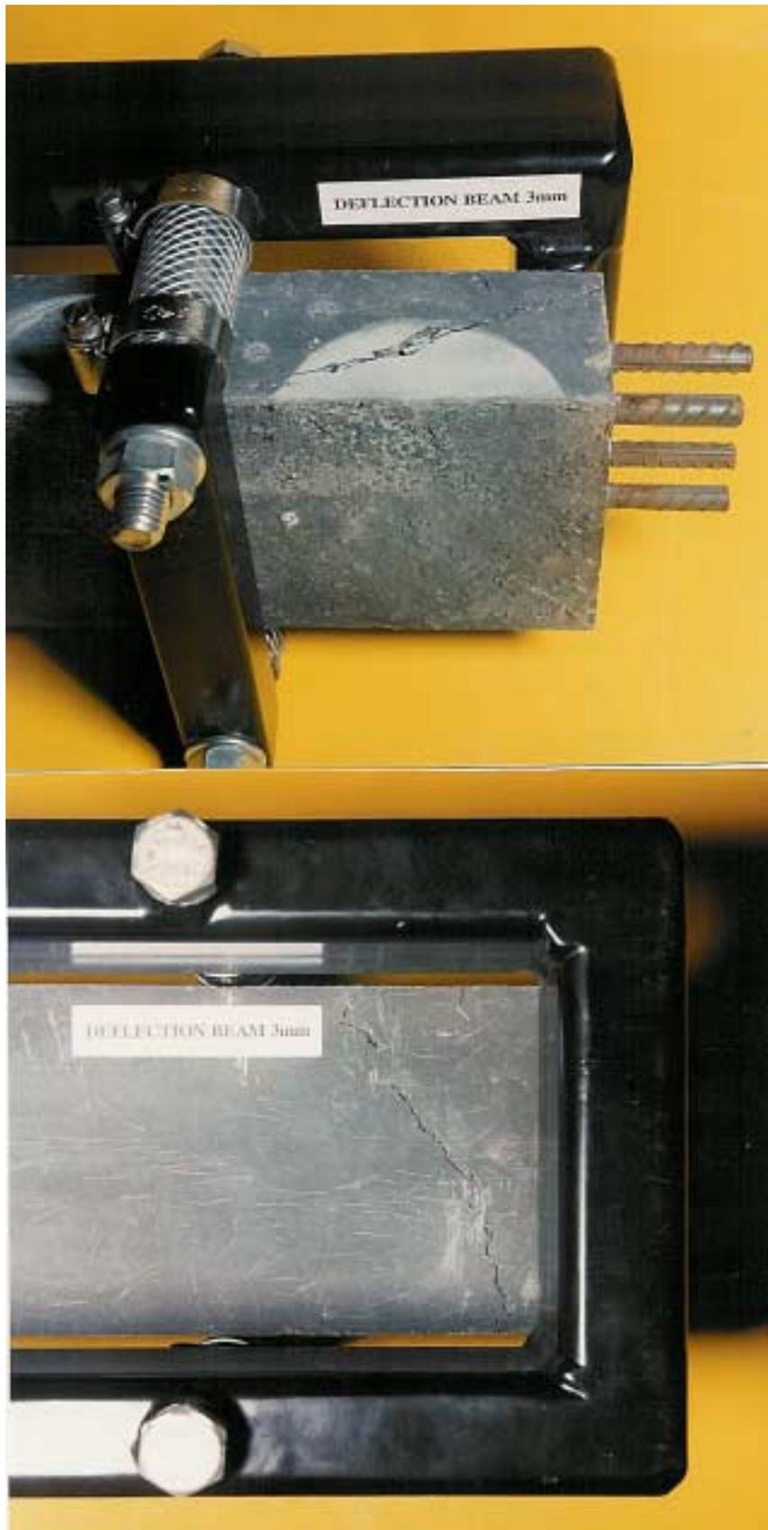
**Figure 4** Beam with center deflection of 3 mm prior to salt water exposure.
