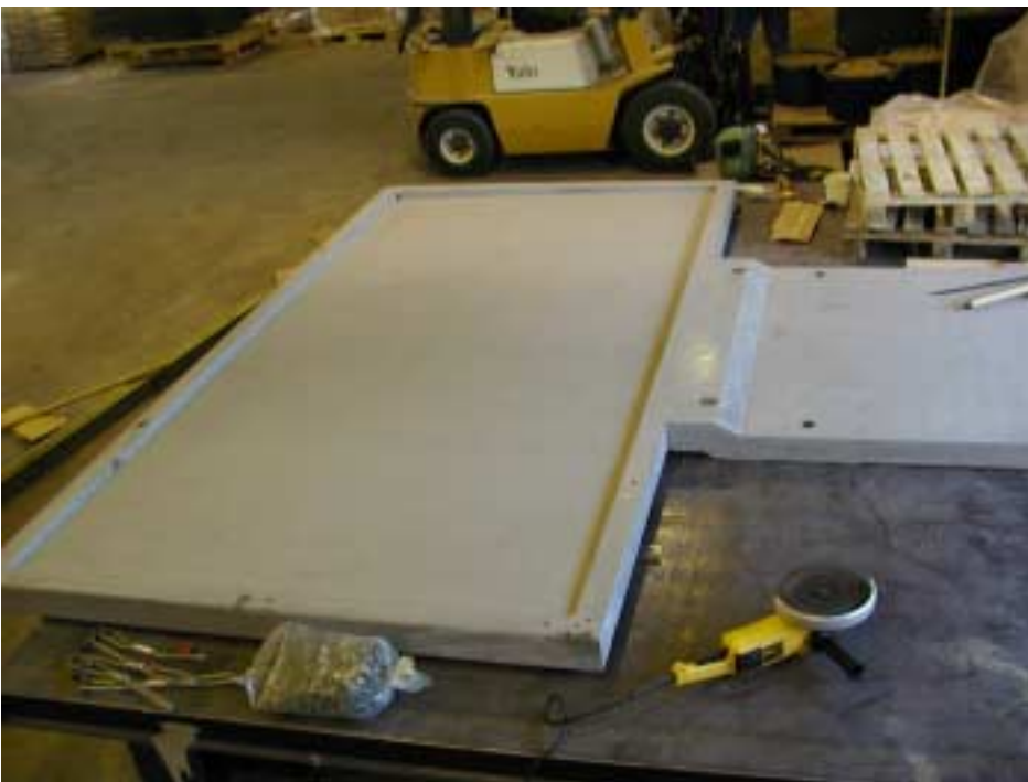
The first of 117 cantilevered balcony slabs for Sandegraven, Vejle in Denmark. The slabs are designed by C.F. Møllers Tegnestue.
