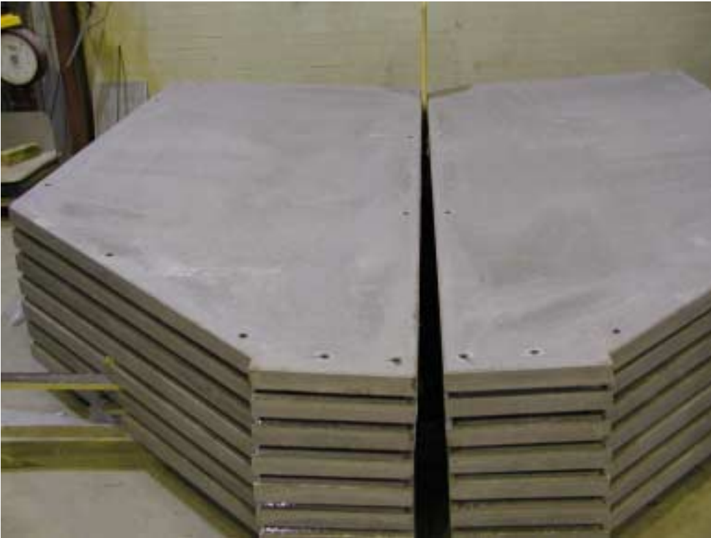
CRC balcony slabs for a retirement home. The slabs are simply supported.
