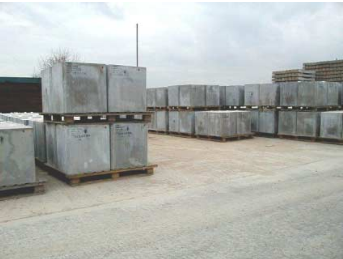
CRC blocks for lining of a mine at Boulby, Scotland. Blocks were produced by Tarmac.
