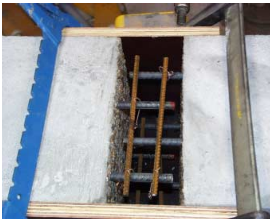
Figure 2 Beam ends with \varnothing 12 mm rebars before the joint is cast with CRC JointCast.
